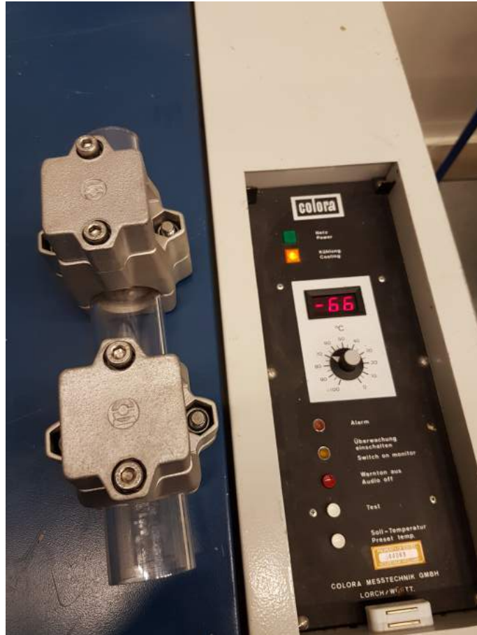
Figure 5.0.1: The big clamps before freezer test
