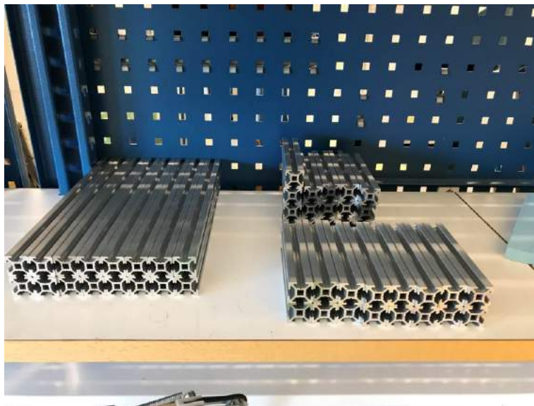
Picture 1: Structural profiles for sensor boxes
