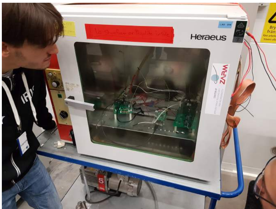
Figure 5.0.4: Electrical system running in vacuum chamber
