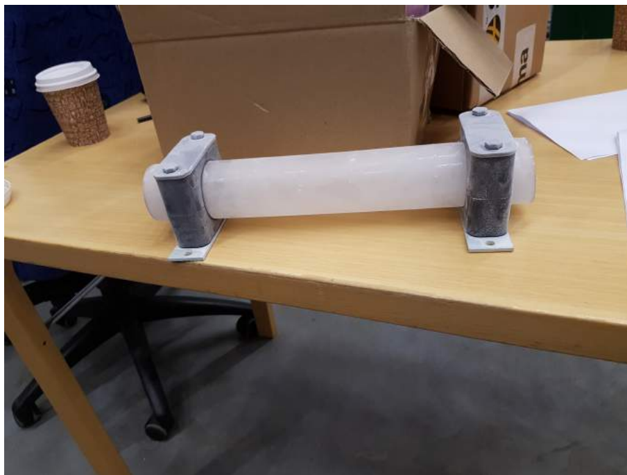
Figure 5.0.2: Small clamps and boom piece after freezer test
